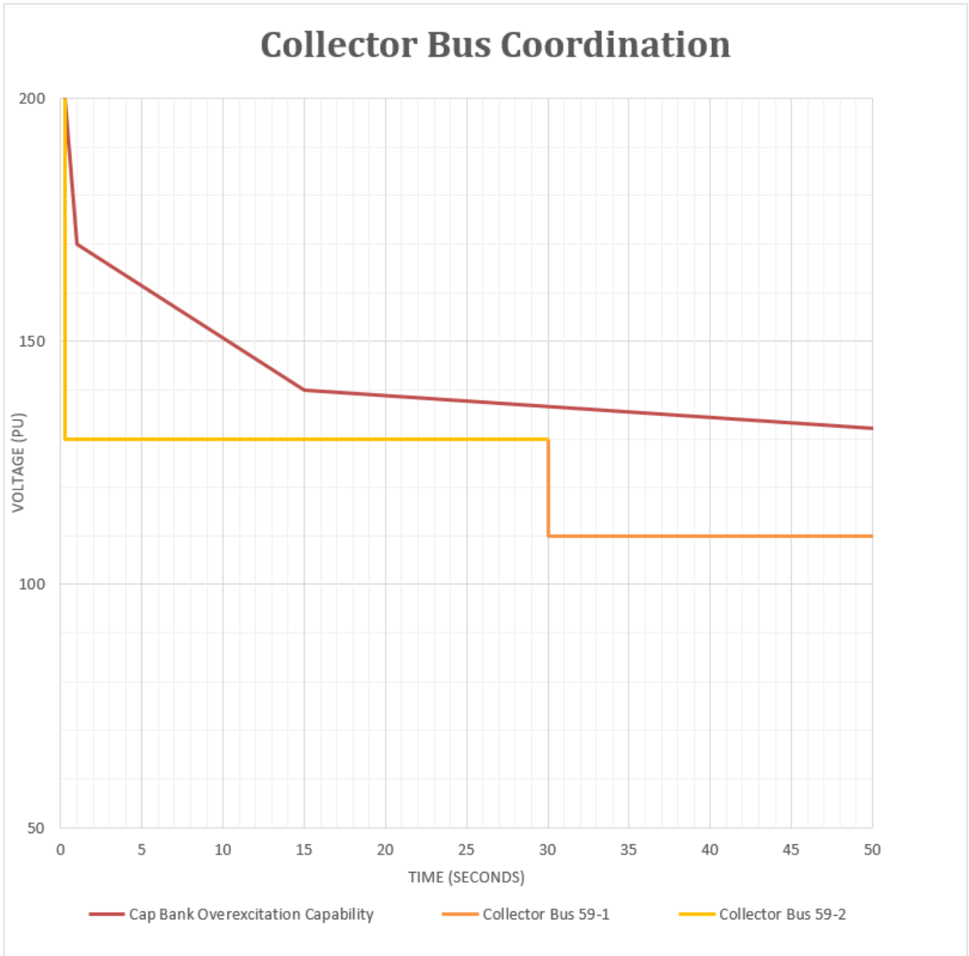
Figure 3.12: Collector Bus Voltage Coordination
